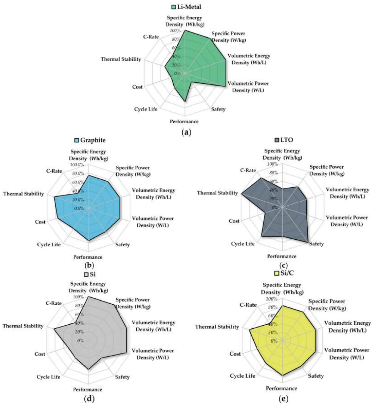
Fig. 16. Performance Comparison of different anode active materials: (a) Li-Metal; (b) Graphite; (c) LTO; (d) Si; (e) Si/C.
