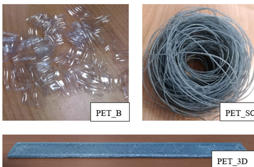
Figure 1. Different processing steps from PET flakes to PET wire and PET 3D sample.
