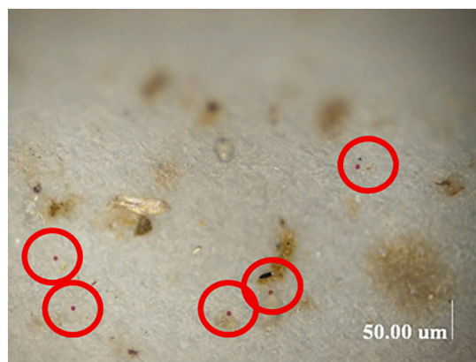
Fig. 2. Red microparticles on filter surface after animal digestion highlighted by rings (C3 = 1.4 particles/mL). (For interpretation of the references to color in this figure legend, the reader is referred to the web version of this article.)
