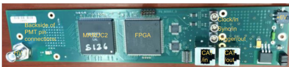
Figure 11. Picture of an FEB module motherboard showing the MAROC2 chip, FPGA, connections for clock, sync, trigger, and the CAT6 daisy-chain. The HV connector for the MAPMT is on the left, and the 6 V connection to power the FEB is on the right.
