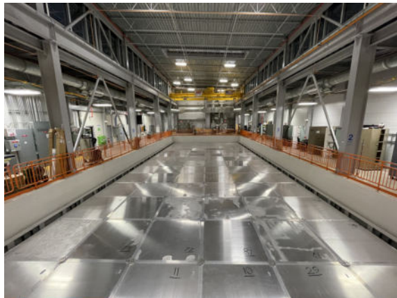
Figure 12. Top CRT horizontal modules installed above the ICARUS detector.
