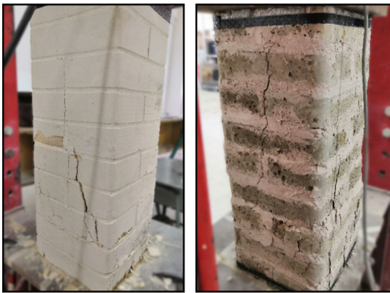
Fig. 7 Crushing typically observed after the C-FRP jacket removal
