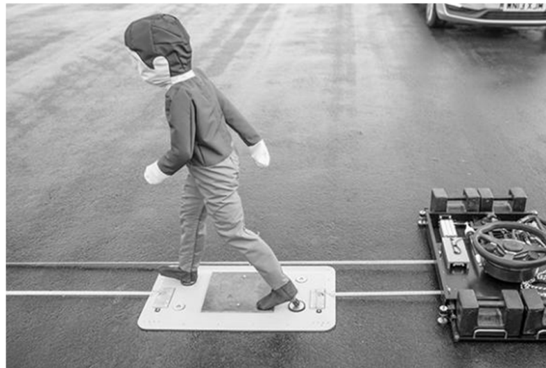
Figure 2. Child soft pedestrian target (SPT) for AEB system tests.
