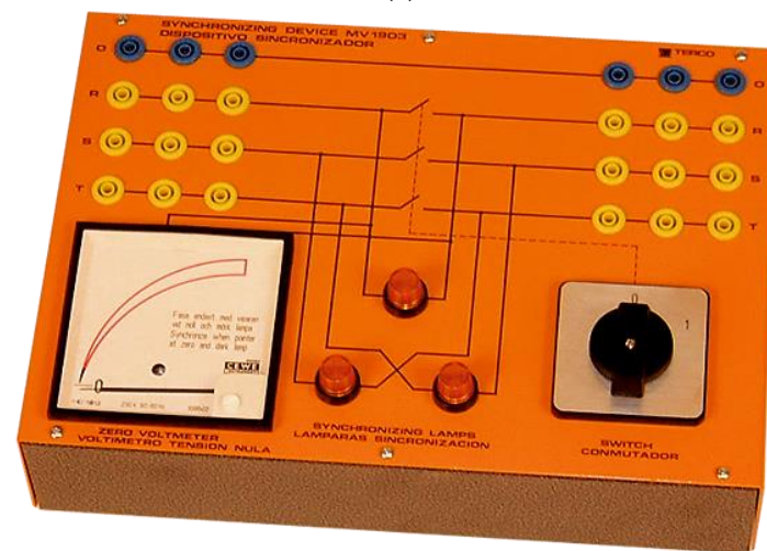
Figure 19. The electrical scheme, as realized in the laboratory for the experimental tests, with the DESG connected to the grid through the synchronization unit (a); image of the used synchronizing device, model MV 1903 manufactured by Terco company, Sweden (b).
