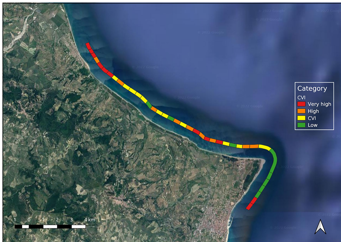
Figure 5. CVI category for each transect. The map was created using QGIS 3.29 software ( https://qgis.org ).
