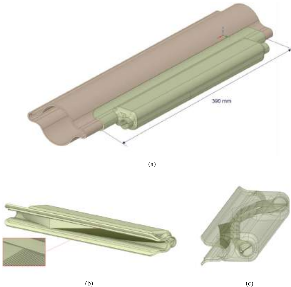
Fig. 3.9 (a) Synchrotron radiation absorber integrated in the vacuum chamber, (b) sawtooth profile highlighted, and (c) cooling channels with twisted tape
