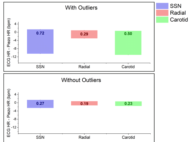
FIGURE 8. Effect of low-quality signal samples on HR estimation. Top: deviation from ECG reference when low-quality signals are included; Bottom: deviation from ECG reference when low-quality signals are excluded
