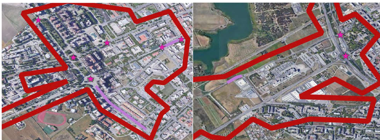
Fig. 4. Examples of identification of segments (violet lines) and intersections (violet points identified by stars) which need safety intervention in the area close to the hospital (delimited by the red line corresponding to the 3 minutes isochrone).
