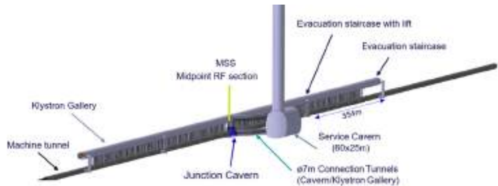
(b) Point PL - 354 m in between staircases
