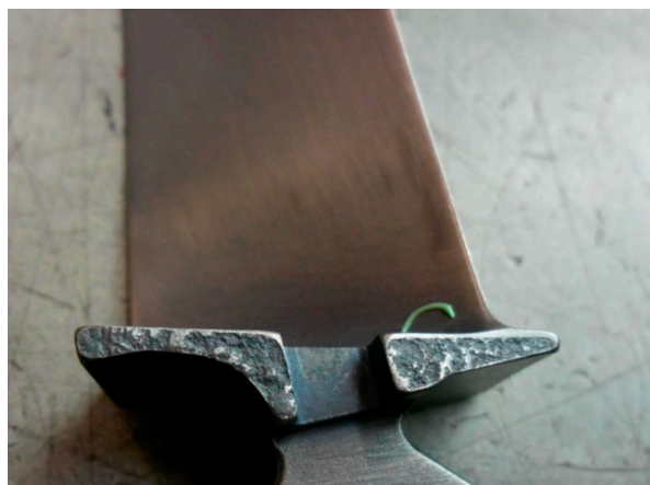
Figure 5. Effect of the abrasion mechanism on a HPC blade [52].
