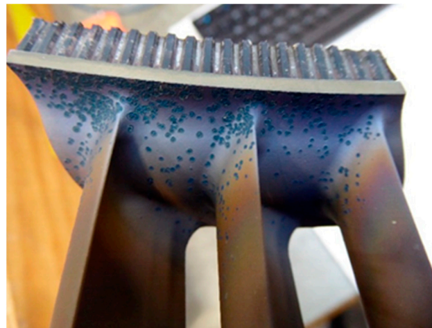
Figure 4. Corrosion effect on a LPT vane [52].
