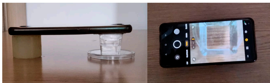
Figure 1. Smartphone-based tracking setup for behavioral analysis of Daphnia magna .
