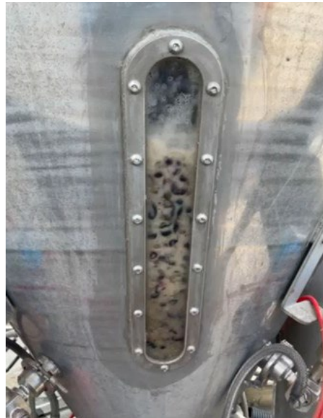
Figure 3. Grape mash mixing with CO 2 in the thermal exchange hopper.
