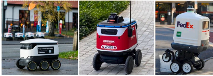
Fig. 1. Autonomous delivery robots examples. From left to right: Starship's robot, Aramex's bot, FedEx Roxo SameDay Bot.
