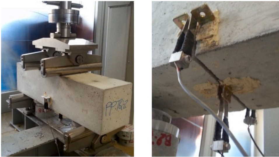
Fig. 4. Test set-up for SFRC specimens.
