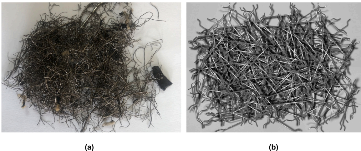
Fig. 1. (a) Waste tyres recovered fibres and (b) manufactured fibres.
