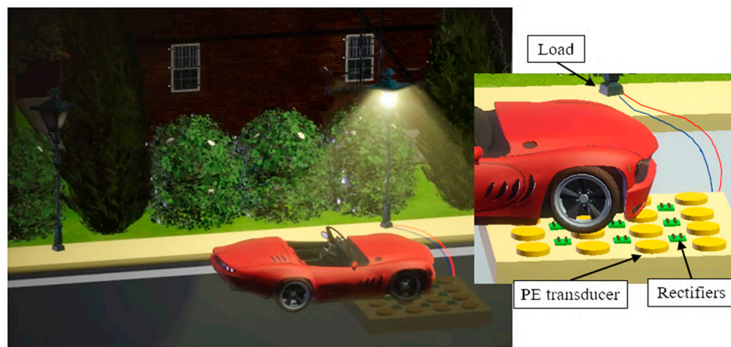
Figure 3. A streetlamp lightened up thanks to the pressure of a car on a slab of PE harvesters.
