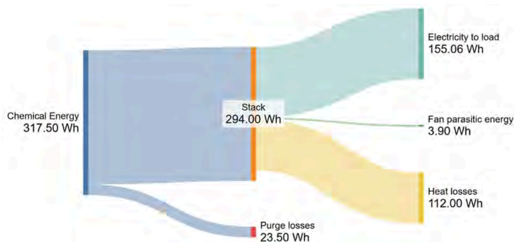
Figure 23. Sankey diagram of the average energy flows in the FCS during the test P2.
