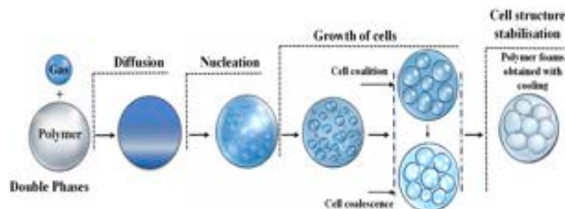
Figure 6. Schematic representation of the microcellular foaming process in polymers, where the lighter shading within the cells indicates a reduced concentration of the blowing agent (Adapted from [131]).
