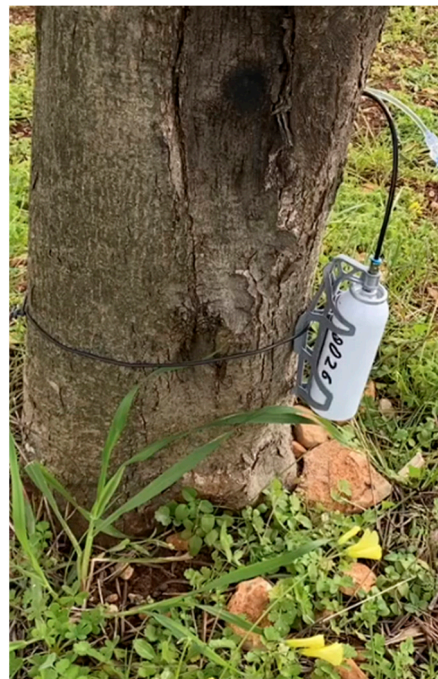
Figure 12. Prototype of Invaio Sciences TIPS™ injection system applied to an olive tree. The system allows a low-pressure release of compounds.
