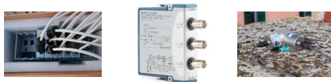
Figure 2. a) CompactDAQ USB with 8 slots; b) NI-9230 module c) Accelerometer blocks
