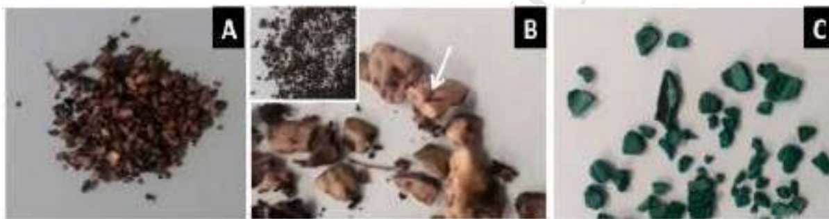
Figure 1: OP a.t camera pictures (A) with related magnification; inset : OP P a.t. (B); OP a.t. loaded with DB dye molecules (C).
