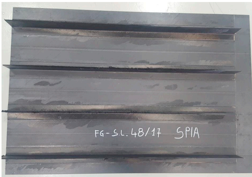
Figure 13. Top view of the stiffened panel manufactured by resin infusion.
