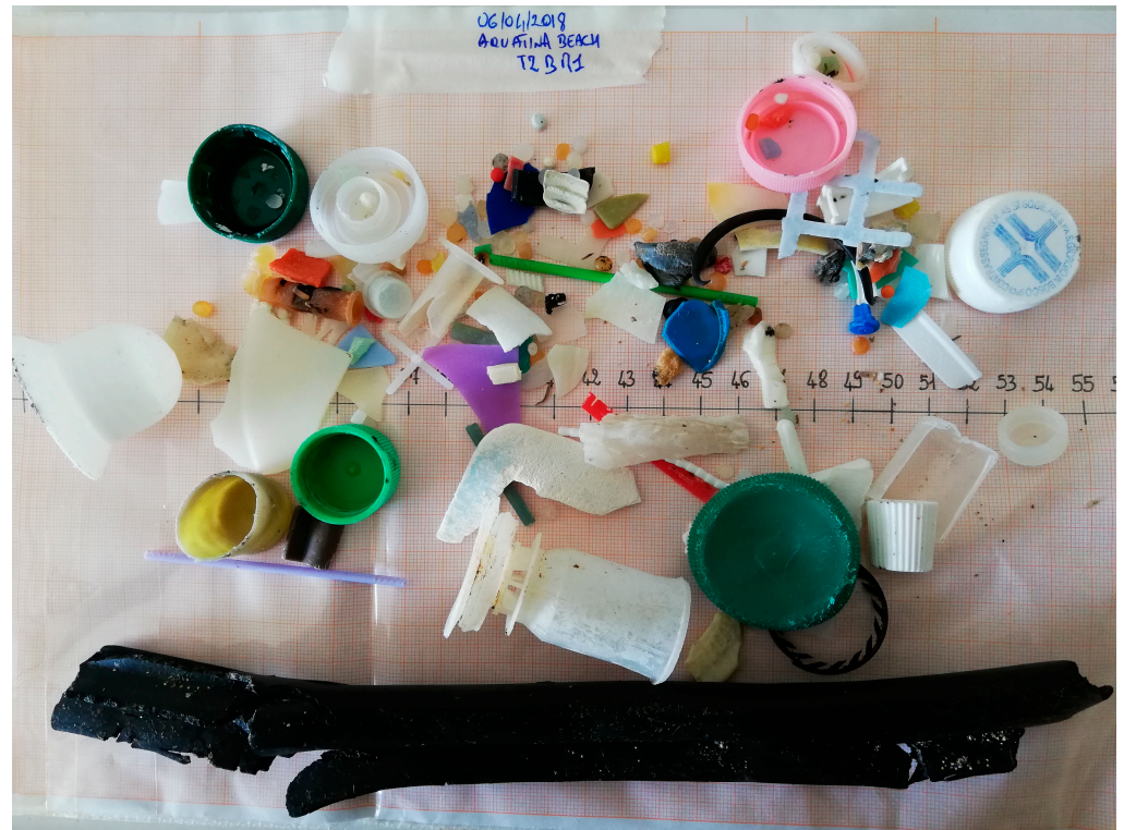
Figure 1. Example of the plastic items collected from Aquatina di Frigole beach. The photo contains the plastic items of a single plot/replicate (sandy beach plot of 30 cm × 30 cm × 10 cm); the label about the sampling time, sampling station and replicate is also reported.
