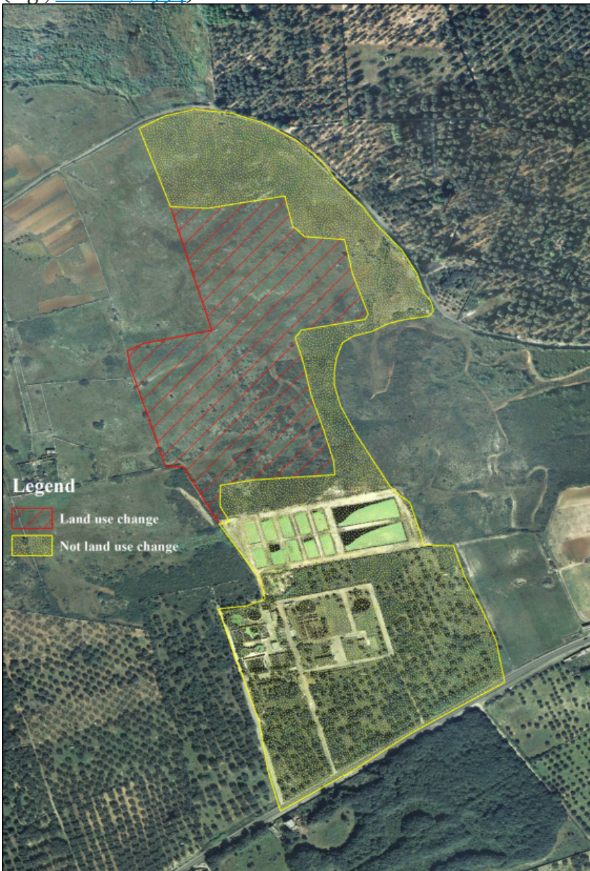
Fig. 3. Orthophoto indicating the area that is changed (conversion of Mediterranean maquis in wetlands) and that is not changed after the construction of the CTW.
