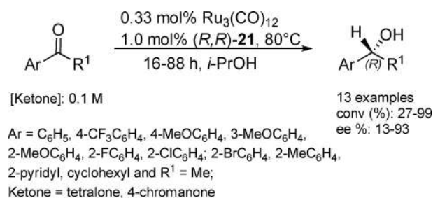
Scheme 12. ATH reactions of a range of ketones carried out in isopropanol as solvent, using the ligand ( R,R )- 21 .
