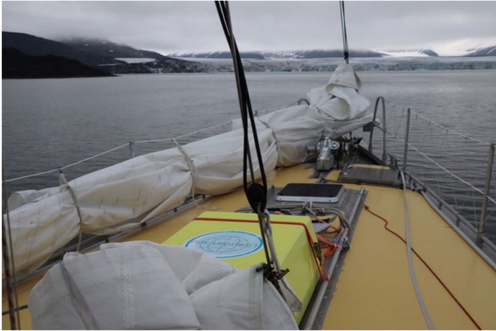
Figure 1: Photo of the POLA-01 detector enclosed in its fiberglass yellow hutch on the deck of the Nanuq sailboat. (Photo by O. Pinazza).
