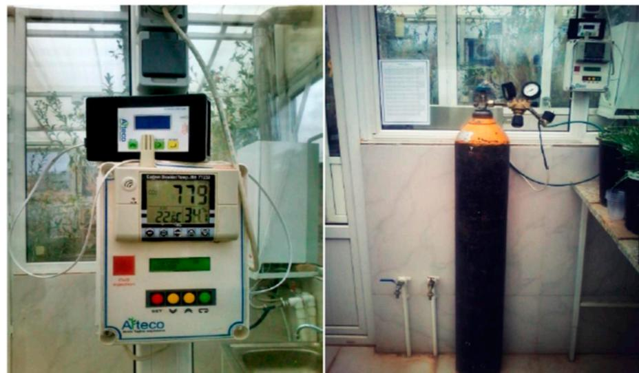
**Figure 1.** Experiment set up. (A) Two-row and six-row barley plant pots under Ambient CO<sub>2</sub> (right) and Elevated CO<sub>2</sub> (left) concentration, just before applying drought stress, (B) CO<sub>2</sub> concentration adjustment device in the greenhouse to apply the CO<sub>2</sub> concentration factor.
